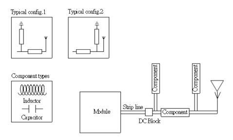
The matching network has to be individually designed using one, two or three components.
