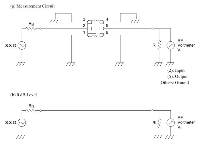
$\label{eq:result} \begin{array}{l} Rg:50\Omega \mbox{ (Internal resistance of S.S.G.)} \\ Ri : 50\Omega \mbox{ (Input impedance of network analyzer or spectrum analyzer)} \end{array}$
