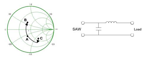
(2) In case of  $R_1 > R_2$  (Real part of SAW impedance is smaller than load impedance)
